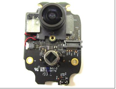
Looking at this PCB, we see one side has a heatsink, and the other side has the Camera Lens,
