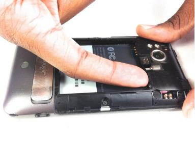
Use your finger to push the MicroSD card in towards the top of the phone, allowing it to be released from the casing.
