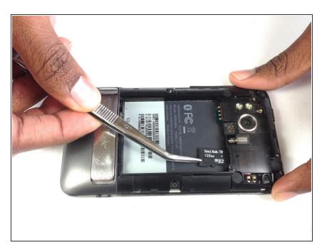
Use tweezers to grab onto the MicroSD card and carefully remove it from the casing.
