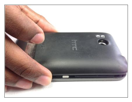
Lift and remove the rear panel.
