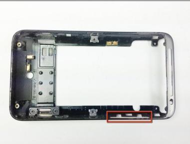
Use a pry tool to lift the buttons out of the case
