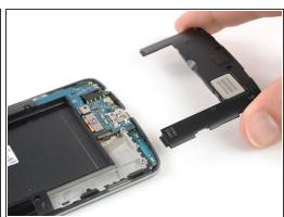
Carefully remove the plastic panel including the loudspeaker by gently pulling it away from the phone assembly.
