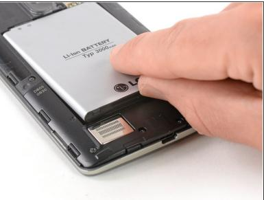
Use a fingernail or a prying tool at the marked notch to lever the battery out of its recess.
