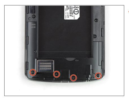
Remove the four Phillips #00 screws (4 mm length).
