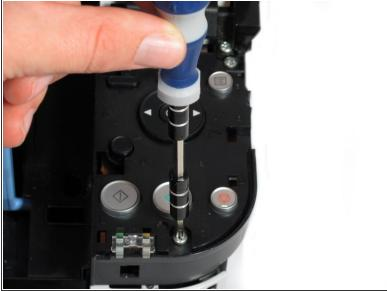
• Remove the five 7.7 mm screws using a Phillips #1 screwdriver.
