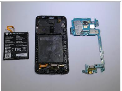
Remove the motherboard assembly from the display assembly with the a spudger or hand.
