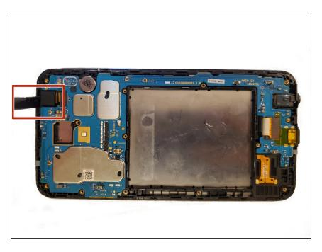
Gently pry out the front-facing camera from the device.
