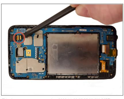
Use the plastic spudger to disconnect the cable connector.
