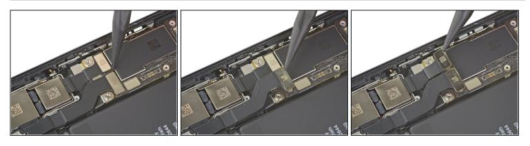
• Use a spudger or a fingernail to disconnect the two camera cable connectors by prying them straight up from their sockets.
