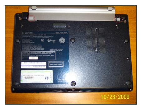
• Remove the battery by moving the 2 release tabs.
