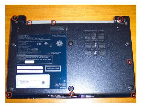
• Remove 8 screws under the computer.
