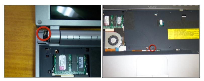
• Remove one screw from top and one from under cap opposite of the power button.
