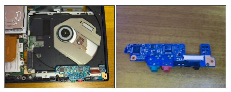
Remove one screw form the sound card. Disconnect one ribbon and one connector (under) from card.
