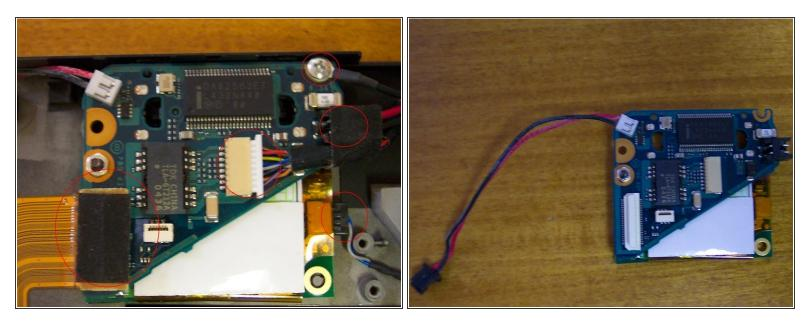
• Remove one screw from the network/modem combo card. Disconnect 3 connectors and one ribbon from cards. There is an additional connector on the motherboard.
