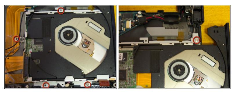
Remove the DVD drive by unscrewing 5 screws, make sure to open the drive with the paper clip to access the last one.
