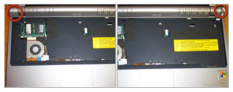
• Remove the power button and cap on opposite side.
