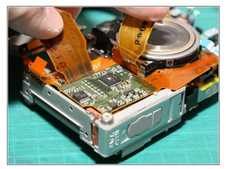
Under the ribbon cables there's another small circuit board. This one is connected to the lens module and appears to contain various motor control chips.
