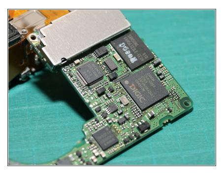
Here's the back of the main logic board. Note the DIGIC chip (main camera processor chip)
