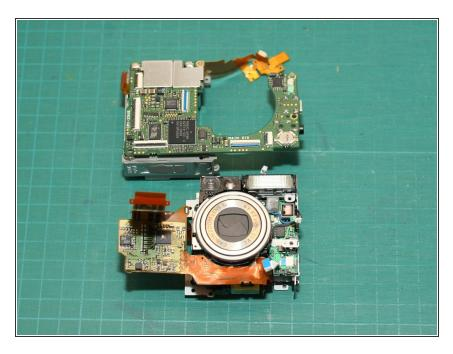
Here's a view of the lens module/viewfinder/flash assembly (bottom) separated from main logic board/battery compartment (top)
