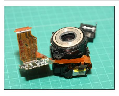
Wait!... not so fast. After reassembling the camera, I found a huge piece of dust on the sensor in all the new images I took. Dust must have entered the lens module during disassembly. I had to take the camera apart completely again! This time, to open up and clean the lens module. :-(
