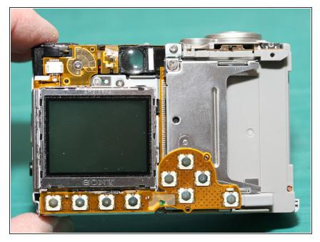
• Here is the back of the camera without the shell. You can see the switch contacts on the flex circuit along the bottom. They're attached to the small metal plate that we'll remove in the next step...
