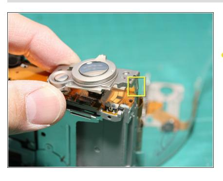
The shutter button can be removed by simply releasing the 2 small catches (one outlined with a yellow square, the other hidden by my thumb)
