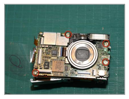
Remove the 4 screws holding the main logic board to the rest of the camera.
