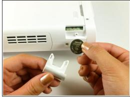
Pull out the battery holder and battery.
