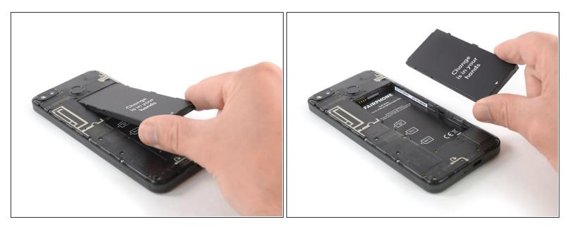
• Lift the battery out of its recess and remove it.
