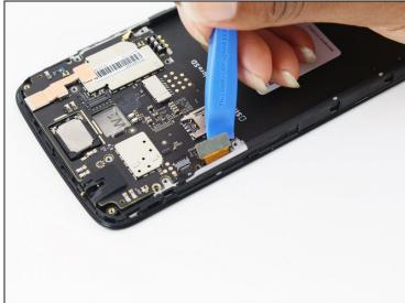
• Disconnect the display cable by prying it straight up from the motherboard.
