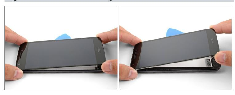
• Lift up the bottom edge of the screen by a few degrees and slice any remaining adhesive.
