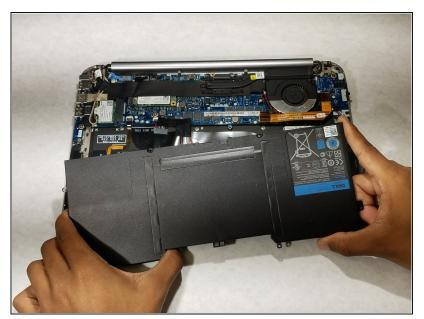
Once all the screws have been removed the battery is now safe to extract
