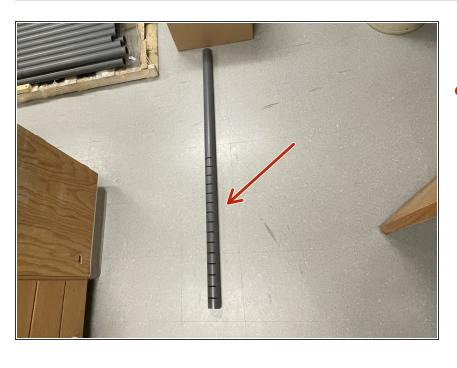
the slits along the 5-ft, 2-inch pipe are cut in the machine shop
