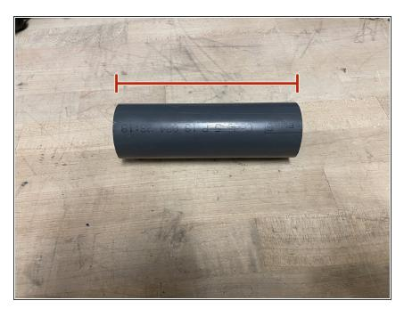
Using the table saw, cut the 1.5-inch pipe to be 6 inches long.
