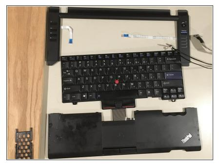
At this point, the only new layout is the shortcut controls, keyboard, and trackpad/wristwrest.
