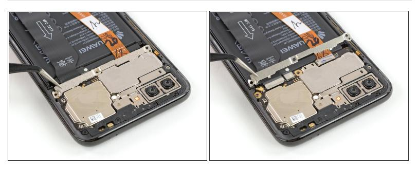
• Use a pair of tweezers to remove the metal shield that covers the connectors of the interconnect cable, the battery and the display flex cable.
