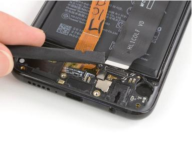
• Use a spudger to pry off and disconnect the bottom end of the interconnect flex cable.
