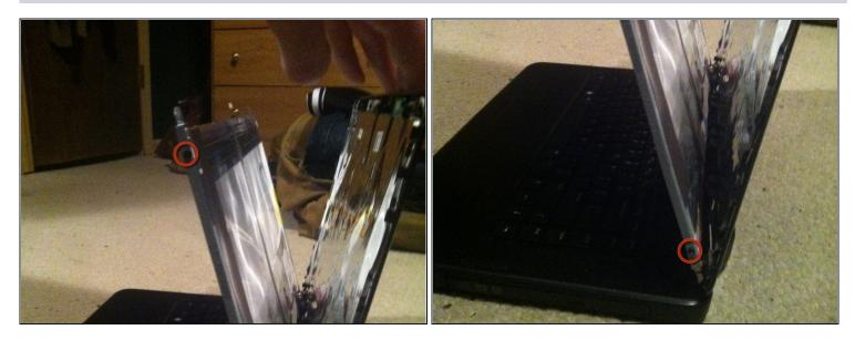
• Now remove the four screws that hold the screen in the metal frame. There are two on each side of the screen.
