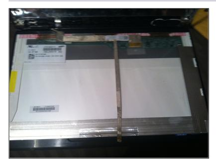
• Once all the screws have been removed and the camera cable disconnected you can lay the screen down on your keyboard to disconnect the other cable.
