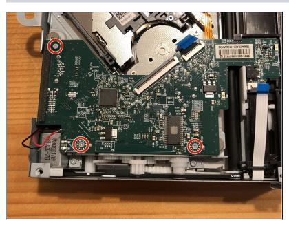
Remove the tiny 3 PH1 screws from the PCB.
