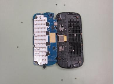
• Remove the six screws marked in red; they hold the keyboard to the sliding mechanism.
