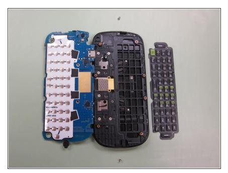
The keyboard ribbon strings each of the pieces together, but the keypad flops right out on its own.
