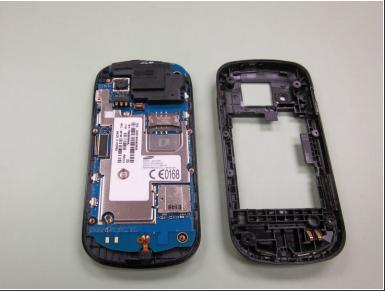
Pry the case away from the body of the phone. Be gentle around the volume control, micro USB, and micro SD ports.
