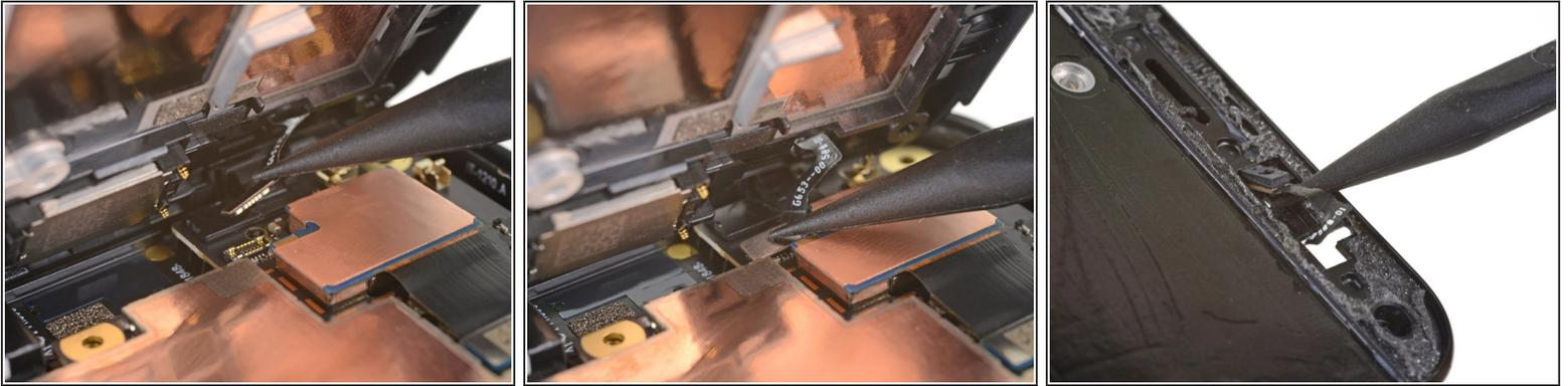
☞ This step shows how to reconnect the proximity sensor during re-assembly.
