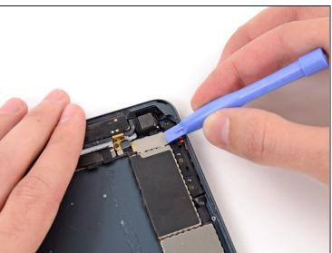
Use a plastic opening tool to push the bracket slightly to the left.
