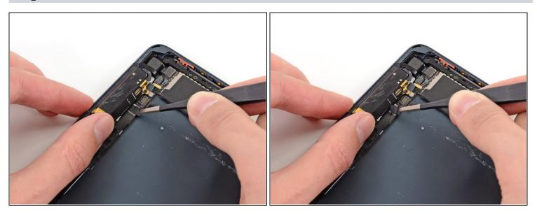
• Use tweezers to peel up and remove the small piece of tape covering the headphone jack cable connector.
