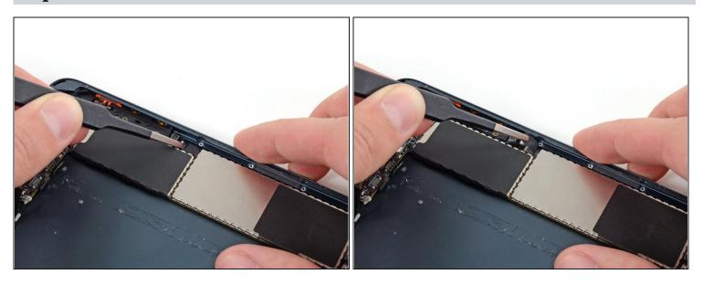
• Use tweezers to peel up and remove the small piece of tape covering the button ribbon cable ZIF connector.
