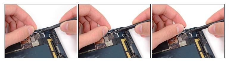
• Use the tip of a spudger to pry the small metal retaining clip off the left antenna cable, then de-route the cable from the clip.
