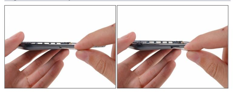
• Use a SIM card eject tool or an uncoiled paperclip to eject the SIM card tray.
