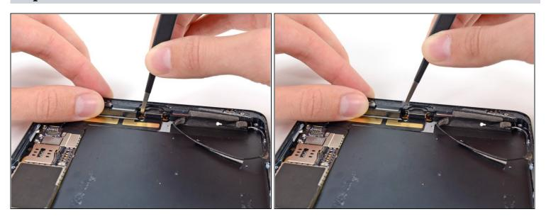
• Use tweezers to remove the small plastic cover on top of the horizontal screw on the right side of the Lightning connector housing.
