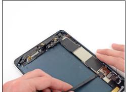
• Gently insert the flat end of a spudger underneath the logic board at various points, slowly prying it up from the rear case.
