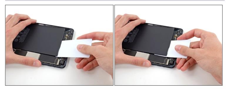
• Remove the plastic card and reinsert it underneath the top right corner of the battery.
