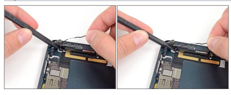
• Use the tip of a spudger to remove the small piece of tape securing the antenna cable in the bottom right corner of the iPad.
