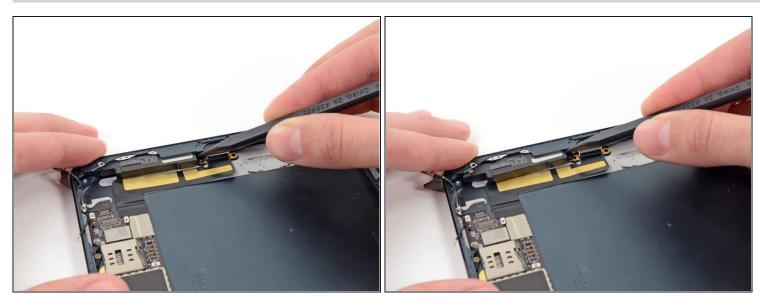
• Use the tip of a spudger to slide the right speaker slightly toward the outside of the iPad.
