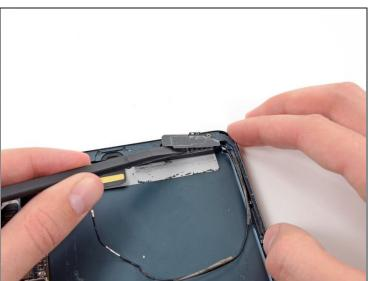
• Use the flat end of a spudger to loosen the foam adhesive securing the lower left antenna to the left speaker.
