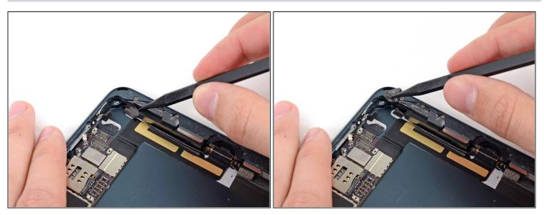
• With the tip of a spudger, peel up the larger piece of tape covering both antenna cables near the bottom of the rear case.
