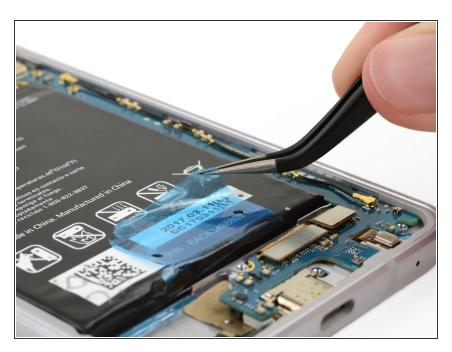
• Use tweezers to lift up the blue pull tab at the bottom of the battery.
