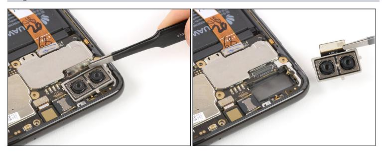
• Use a pair of <u>tweezers</u> to remove the rear cameras.
