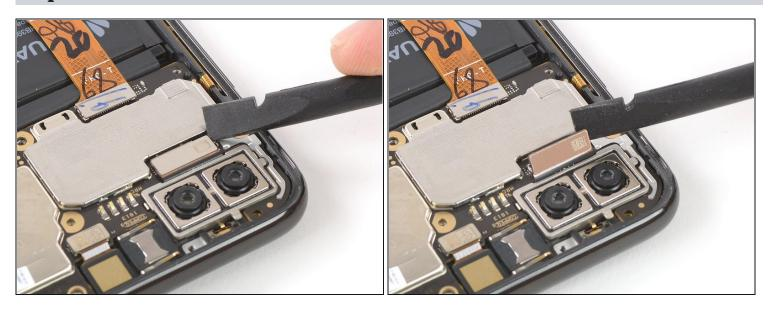
• Use the flat end of a spudger to pry up and disconnect the flex cable for the rear cameras.
