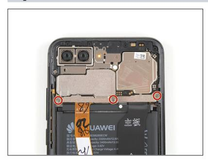
Remove the three Phillips #00 screws (2.9 mm length) that secure the metal bracket on top of the battery, interconnect, and display flex cable.
