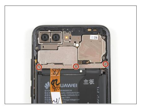
Remove the three Phillips #00 screws (2.9 mm length) that secure the metal bracket on top of the battery, interconnect, and display flex cable.
