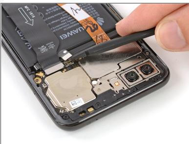
Use a spudger to pry up and disconnect the battery flex cable.
