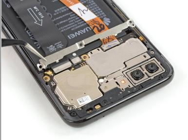
• Use a pair of tweezers to remove the metal shield that covers the connectors of the interconnect cable, the battery and the display flex cable.
