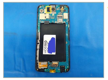
Use a Halberd spudger or an opening pick to disconnect the front camera flex from its connector on the motherboard.
