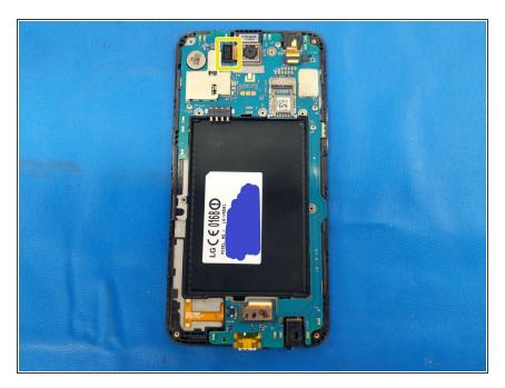
Use a Halberd spudger or an opening pick to disconnect the front camera flex from its connector on the motherboard.
