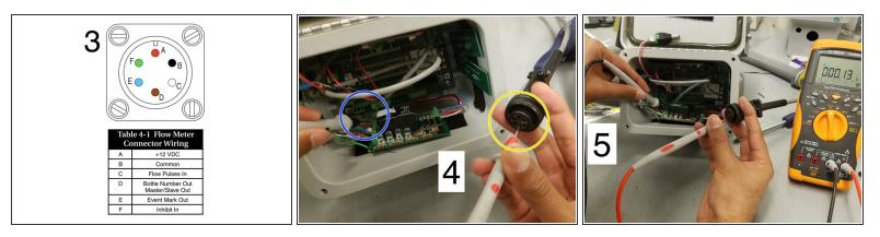
A Be sure not to cross the leads when testing a wire so as to not short the wire!
