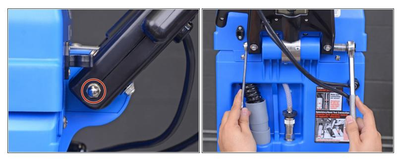
Use a 7/16" (11 mm OK) wrench to hold the handle axle while you use a 7/16" socket to remove the cap nut securing the axle end.
