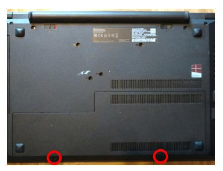
• Remove the two screws at the back bottom.
