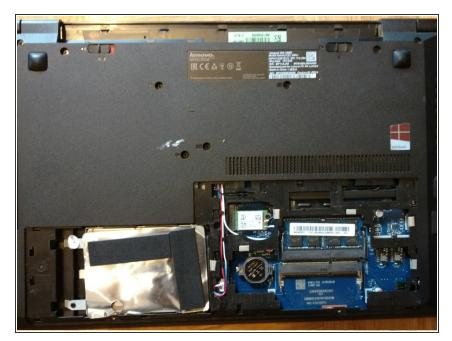
Remove the back cover by sliding it out.
