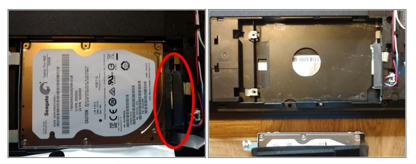
Disconnect the harddrive connector by sliding it left. Then remove it.
