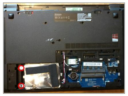
• Remove the two screws that attach the harddrive to the laptop.
