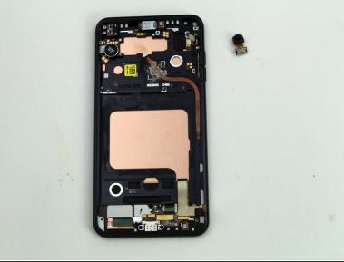
Use a Spudger to pry away the front-facing camera from the board.
