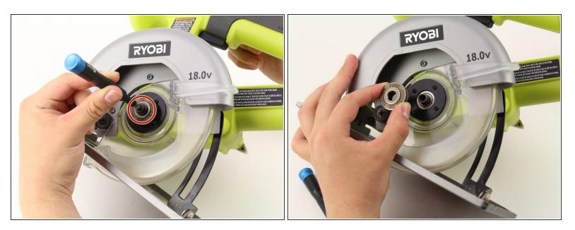
Unscrew clockwise and remove the bearing in the middle, connecting the blade to the motor. This will also allow removal of the blade guard.
