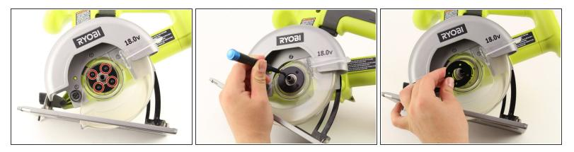
Remove the four black screws holding the black bearing and remove the bearing itself.
