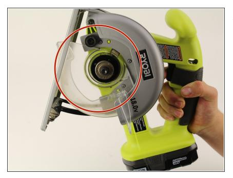
Locate the area where the blade is connected to the motor, where the circular covering is on the Ryobi P501G.
