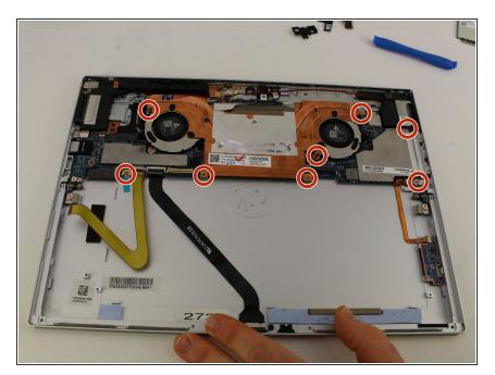
Use the Phillips #00 Screwdriver to remove the eight 2 mm screws.
