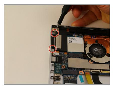
Unscrew the two speaker/antenna module mounting 2mm screws using a Phillips #00 Screwdriver.
