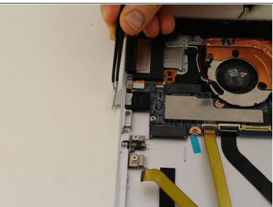
Remove the SD Card holder from the motherboard.
