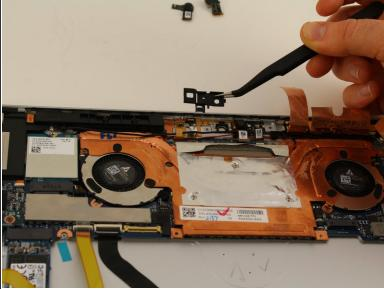
Using tweezers or your fingers, lift up and remove the plastic covering and set it aside.
