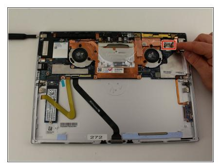
Undo the two small connectors by pulling gently.
