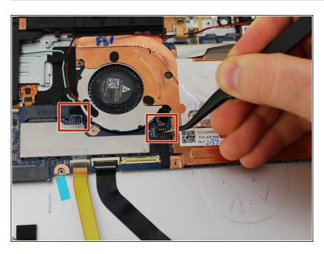
Undo the two indicated connectors near the fan using your fingers or tweezers.
