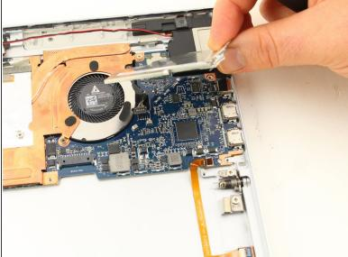
• Lift up the flap on the right of the indicated plate, and lift the whole covering off.
