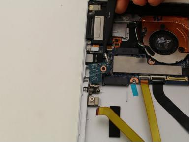
Unscrew the single 2mm screw from the peripheral board with the same screwdriver, and remove the peripheral board from the motherboard.
