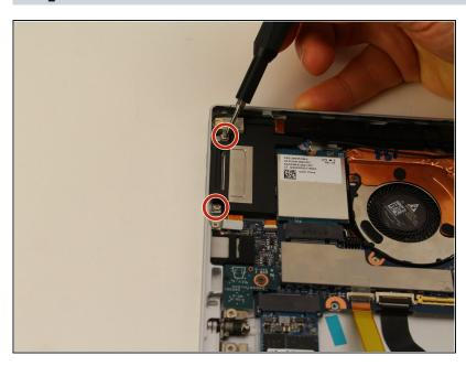
Remove the two speaker/antenna module mounting 2mm screws using a Phillips #00 Screwdriver.
