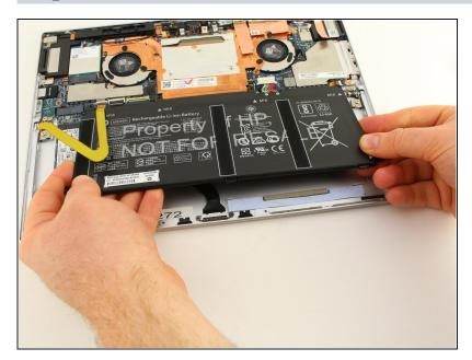
• Lift the battery out of the housing.
