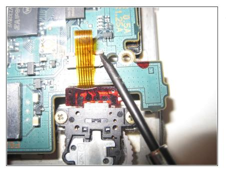
Next, use your screwdriver to lift up on the connectors that connect the scroll wheel to the circuit board. Then pull out the ribbon.
