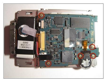
This part of the tear-down proved to be the most frustrating. BE AWARE THAT THE 5 SCREWS CIRCLED WERE EXTREMELY TIGHT! I actually stripped out my cheapo #0 Phillips screwdriver. These 5 screws must be removed to separate the screen from the circuit-board. At this junction I think I am supposed to reveal the technical aspect of what I have found on the circuit board. Unfortunately I see nothing remarkable. There is a Dragonball
