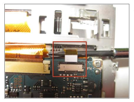
• The next step involves separating all of the various ribbon wires from the screen and circuit board. There are 5. The first wire is the ribbon wire that connects the memory card to the circuit board. I pulled it out with my screwdriver like shown but I am sure that black piece of plastic piece could have been moved to release the wire from the connectors mighty grip.
