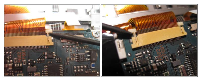
Next I removed the wide ribbon that connects the interface to the circuit board. Lifting up on either side of the connectors two white tabs releases the ribbon.
