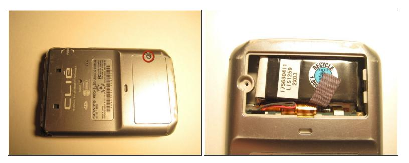
• The next thing you'll want to do is remove the battery compartment screw. No need to take the battery out yet. That little bugger comes out easier after the outer frame comes off.
