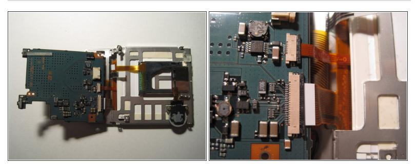
Next, flip the board over so you can see the back side. There should be 3 ribbons attached to the circuit board. (In the picture the white one was not attached as it easily came out when I flipped the board over.) Remove these ribbons from their connectors by simply pulling them out. The circuit board should fully separate from the frame holding the screen now.
