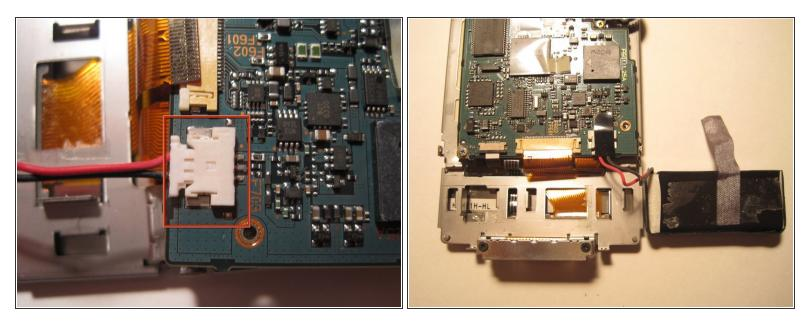
• Next, remove the battery. Simply find the red and black wires where they meet the connector on the circuit board. Remove the black tape, grasp the connector near the wires and pull. Easy enough.
