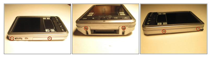
• The first thing you will want to do to tear this mother down will be to remove the 6 screws around the three sides of the unit. This requires the #0 Phillips screwdriver.
