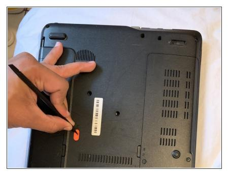
Using a nylon spudger or your fingers, push down on the battery clip to release the battery.
