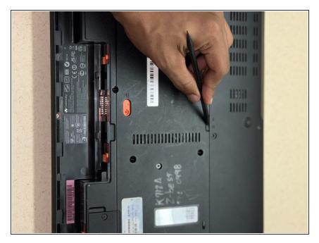
Locate the casing that protects the RAM modules, wireless card, and hard drive.
