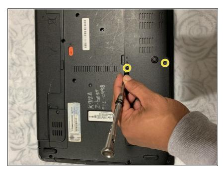
With the PH1 head from the tool kit and the adjustable screwdriver, remove the 2 M3x5.0mm screws on the casing to get to the RAM modules.
