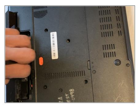
Finally, remove the battery by detaching it from the laptop casing.
