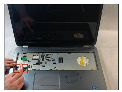
Using your fingers, unplug the two palmrest ribbon cables found at the bottom left of the integrated keyboard's slot.
