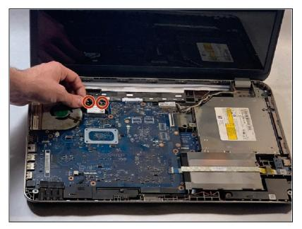
Disconnect the two antenna cables connected to the WLAN card.
