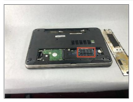
Pull each RAM stick out of the machine, separating each piece from its respective slot.
