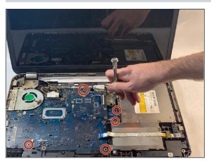
Using a Phillips screwdriver, remove a total of five screws (two 3mm, five 5mm) from the locations marked on the image.
