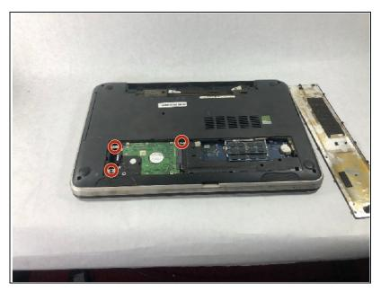
Using a Phillips #000 screwdriver, remove the three 5 mm screws securing the hard drive to the laptop.
