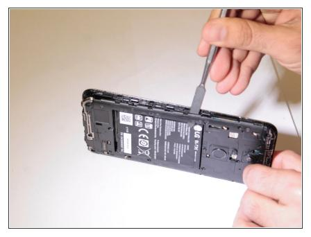
• Use a metal spudger or plastic opening tool to pry open the outer cover.
