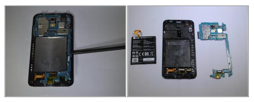
• Remove the motherboard assembly from the display assembly with the a spudger or hand.
