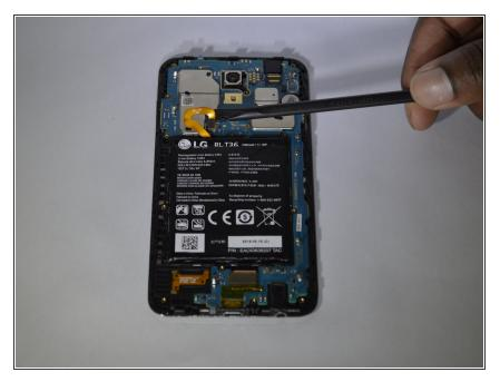
• Use the flat end of a spudger to detach the battery connector from the logic board.
