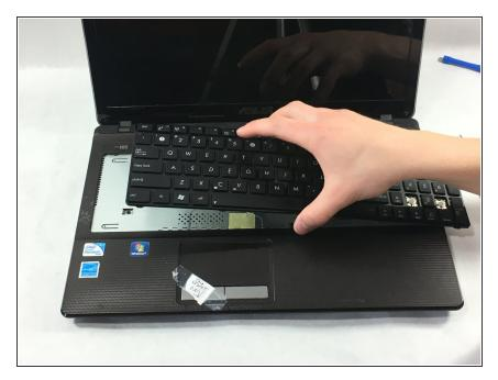
Carefully disconnect the "bus" connector from the laptop. Press on it with your thumb/index finger and slide it right along the surface of the laptop.
