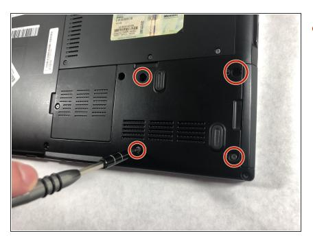
Remove the four 3.0mm Phillips #1 screws securing the hard drive casing.
