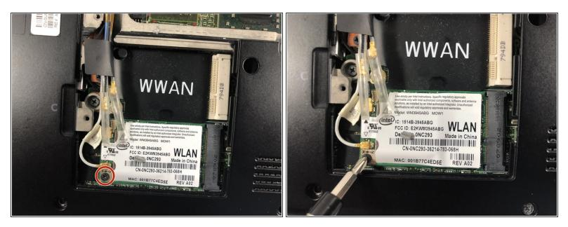
Unscrew the 3.0mm Phillips #1 screw from the wireless card.
