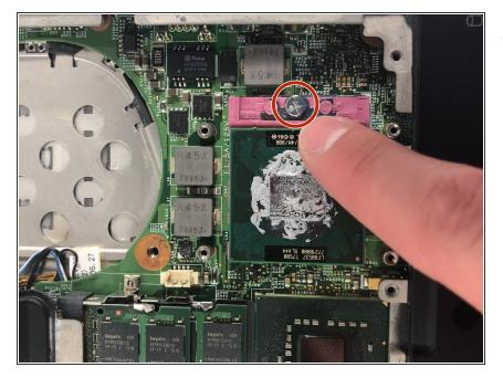
Using the flathead screwdriver, turn the one screw counterclockwise to loosen the CPU, but do not remove the screw.
