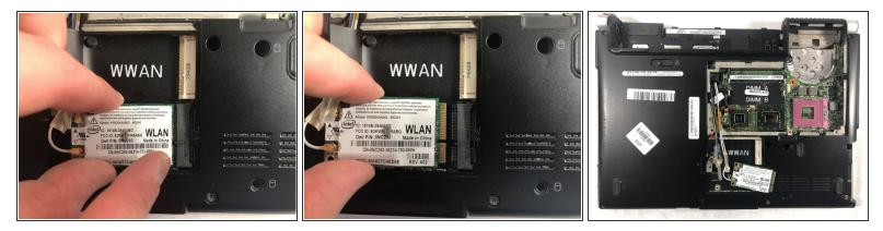
• Slide the card to the left and up to remove it.
