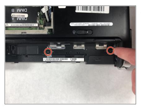
Remove the two 2.5mm Phillips #1 screws in the battery housing port.
