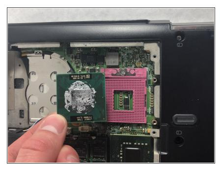
• Carefully lift the CPU away from its housing.
