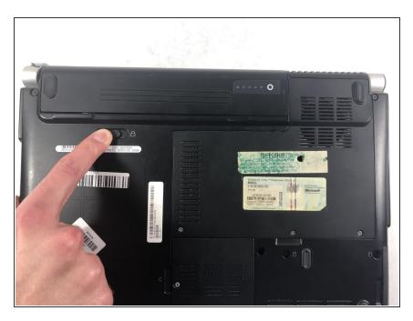
• Push and hold the slide button to the left and unlock the mechanism.
