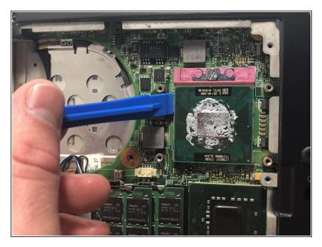
• Using the iFixit opening tool, prop up the CPU.
