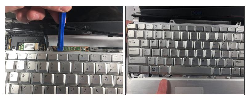
Mhen removing this piece lift slowly as there is a cord underneath that connects to the keyboard.
