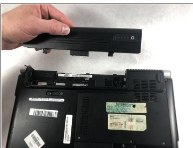
Lift the computer up and slowly pull the battery straight out from the device.
