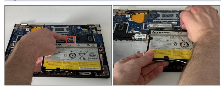
• Grip the base of the connector with your fingers or pliers, and gently pull the connector straight back towards you to remove it.
