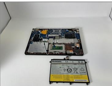
Carefully remove the battery from the laptop.
