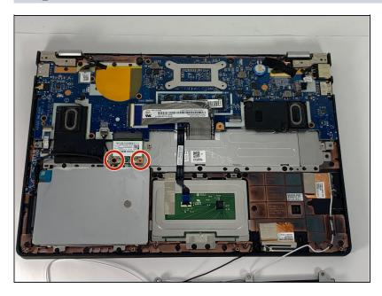
Use the Phillips #000 screwdriver to remove the two 3.3 mm screws.
