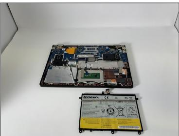
• Carefully remove the battery from the laptop.
