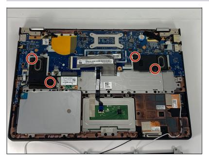
Use the Phillips #000 screwdriver to unscrew the four 1.7 mm screws.
