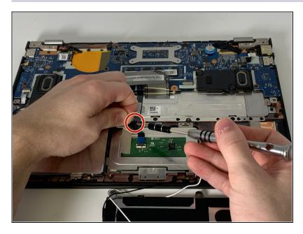
The eighth screw at the top left is covered by a piece of silver tape. Gently peel the tape back and remove the screw.
