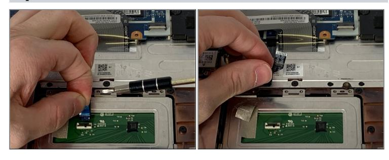
• There is a blue plastic tab connected to the cable. Use this to gently pull the cable directly back and out of the connection point on the touchpad. If the black tab has been unlocked this should slide out without resistance.
