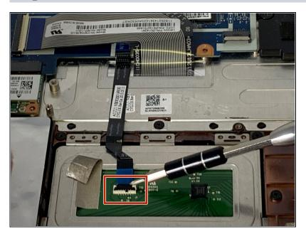
There is a small black tab holding the cable for the touchpad in place. Flip this tab up using a nylon spudger to unlock the connector.
