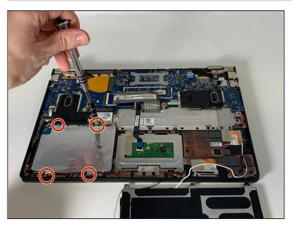
Use the Phillips #000 screwdriver to remove the four 3.3 mm screws securing the hard drive to the panel.
