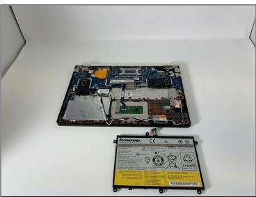
Carefully remove the battery from the laptop.
