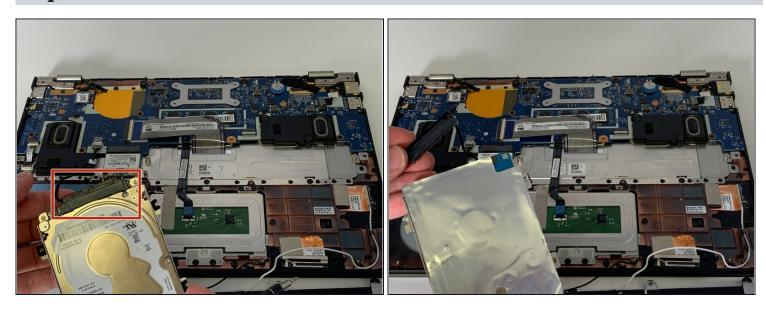
• Lift the hard drive up, turn it over, and remove the connection.
