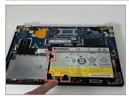
Gently remove the three pieces of tape securing the Bluetooth/Wi-Fi antenna.
