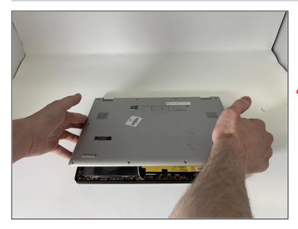
• Carefully remove the back panel by gently separating the panel from front to back.
