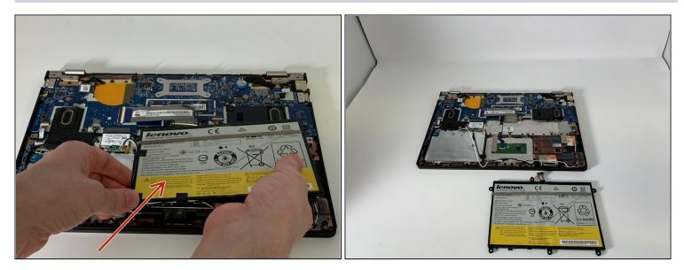
• Carefully remove the battery from the laptop.
