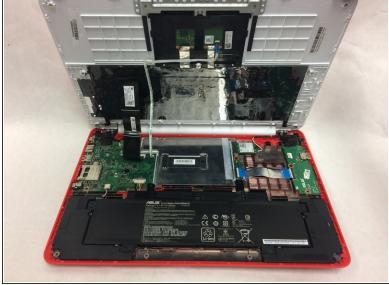
Fully separate the plastic case from the keyboard by lifting it upward.
