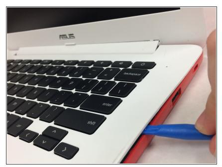
Separate the plastic case from the keyboard at the seam using a plastic opening tool.
